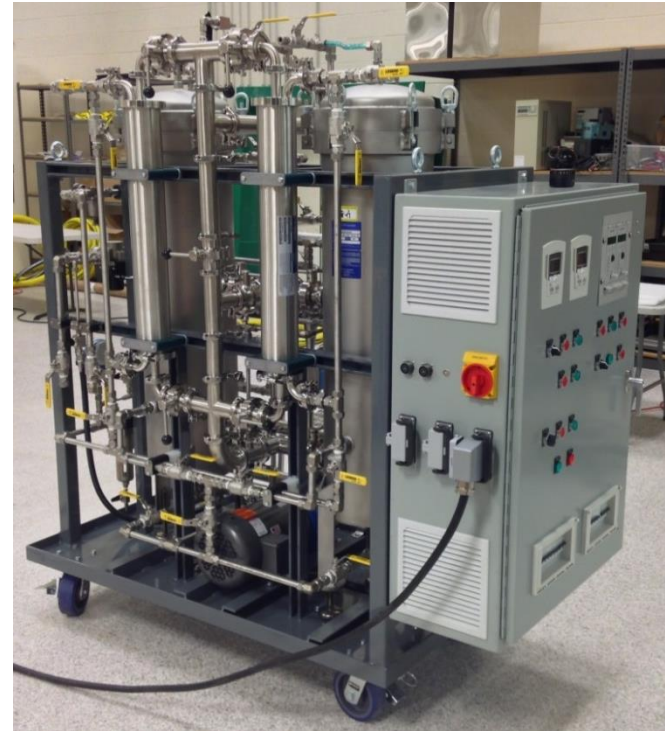
Lower UEC controls: level, temperature, dissolved gas, particle filtration, transducer on/off
